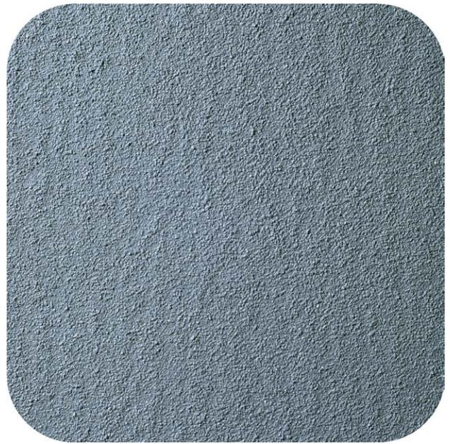
**Figure 1.** This photo illustrates the appearance of 20% SoftSand Gray particles in a gray paint. The particles were mixed into the paint and applied by a roller.
