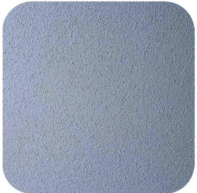
**Figure 2.** This photo illustrates the appearance of SoftSand Gray particles that were sprinkled onto a gray paint. A top coat of gray was applied after the first coat (with the particles) had dried.
