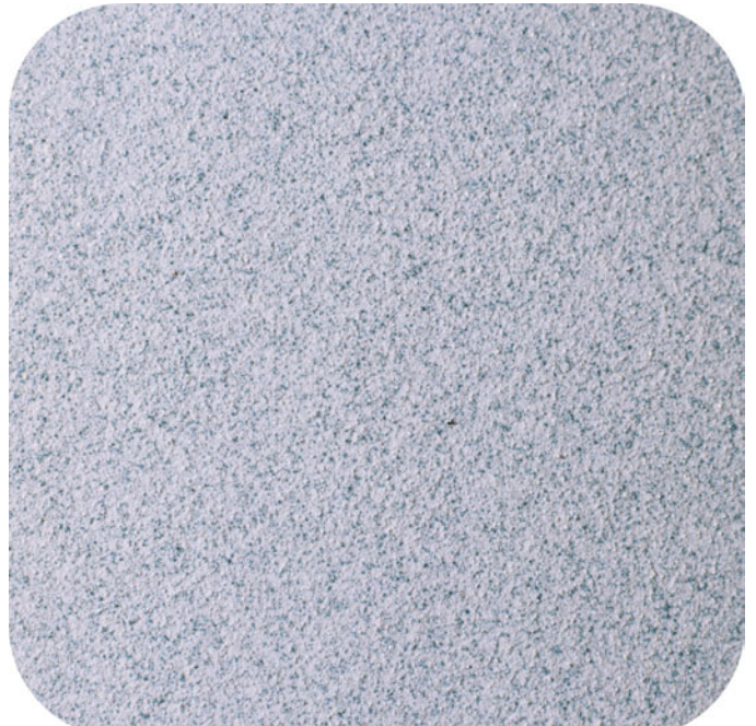
Figure 2. This photo illustrates the appearance of 20% SoftSand Seafoam Green particles in a white acrylic paint.
